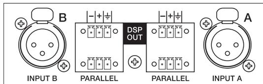
The inputs INPUT A & INPUT B are electronically balanced offering an input sensitivity of +6dBu (1.55V) for direct connection of mixing consoles, etc. Connection can be established via the XLR-type input connectors or the supplied screw-on connectors, which are connected in parallel. The pin-assignment of the XLR-type input connectors is according to the
